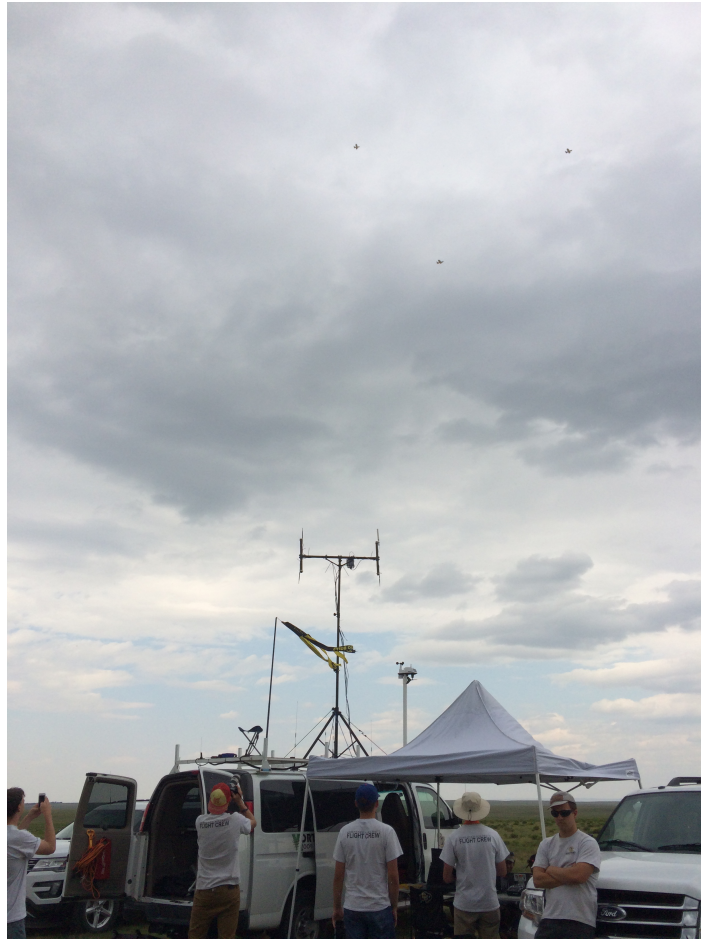
Figure 5.3: Image of the ground station antenna used for the 2.4GHz C2 link during summer 2017 flights for KAIST.
